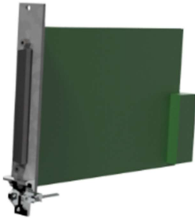
Figure 10 PXI instrument ready for DAK attachment
