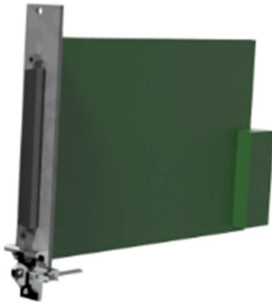
Figure 10 PXI instrument ready for DAK attachment
