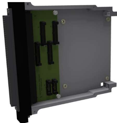
Figure 3 Primary PCB is now visible.
