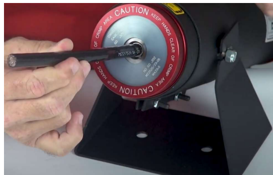
Fig. F. (Contact and wire in Crimp Tool)
