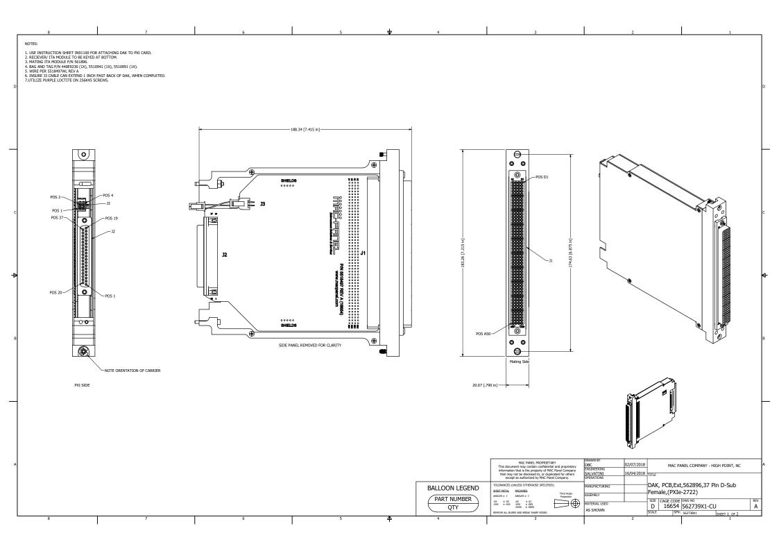
NOTES: 1. USE INSTRUCTION SHEET IN91100 FOR ATTACHING DAK TO PXI CARD. 2. RECIEVER/ ITA MODULE TO BE KEYED AT BOTTOM. 3. MATING ITA MODULE P/N 561896. 4. BAG AND TAG P/N 440E9230 (1X), 5510941 (1X), 5510991 (1X). 5. WIRE PER 5518497WL REV A
