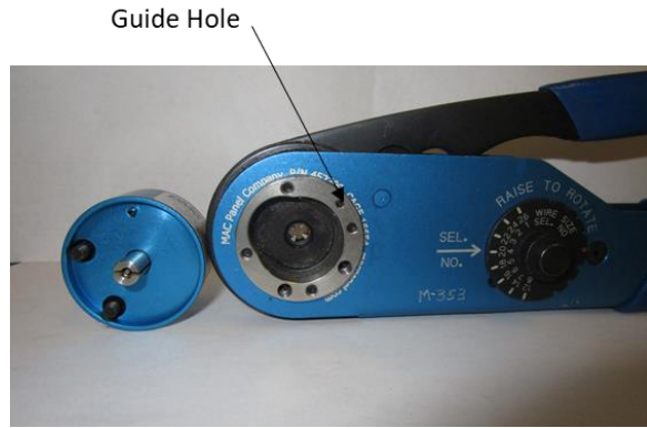
Detail A. (Positioner and Crimp Tool)
