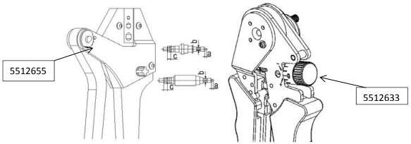
4. Crimp the strain relief part of the contact, approximately 4 mm (c) long from the cable jacket, using the FO crimping tool. When crimping the strain relief, make sure the contact is positioned in SW 3 mm cavity. 5. The protruding fibre is polished by means of a polishing block (7 mm depth) with grain size 1000. Make sure polishing is performed on a flat and solid surface. The very tip of the contact can be polished with a  $9\mu$  grain size polishing paper.
