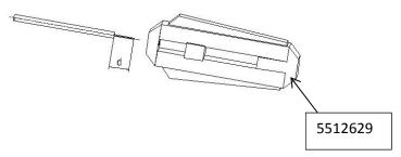
2. Insert the stripped POF cable into the proper contact. Make sure the fiber protrudes 1 mm (a) out of the contact. For the female contact the barrel has to be screwed off in beforehand.
