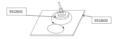
6. The barrel has to be screwed onto the female contact. Make sure that the snap ring has the correct position.
