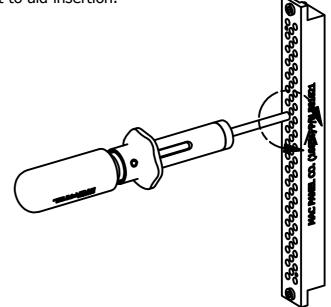
Step 2) Depress plunger to extract contact. Whilst keeping the end of the Extraction tool pressed against the module. The contact will be pushed out of the rear of the module.
