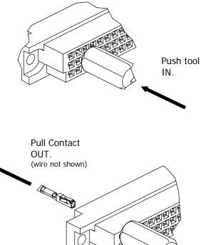
Keeping pressure on the extraction tool to keep the locking lance depressed, Gently pull the wire and contact out from the BACK of the receptacle.
