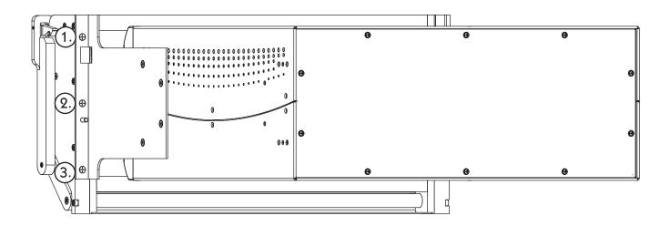
Step 4. Illustration of completed receiver mounted to flanges.
