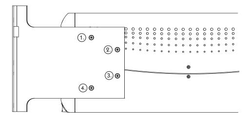
Step 2. Illustration of completed flanges mounted onto PXI chassis. Notice notch for safety switch on right side flange.
