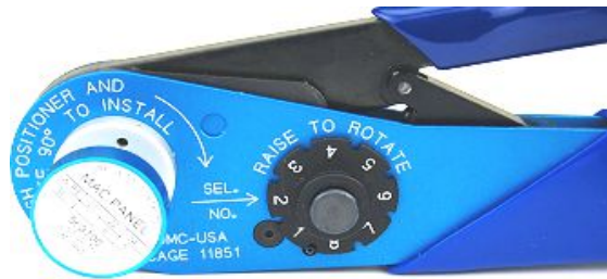
Fig. D. (Positioner inserted into Crimp Tool)
