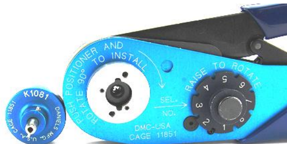
Detail A. (Positioner and Crimp Tool)
