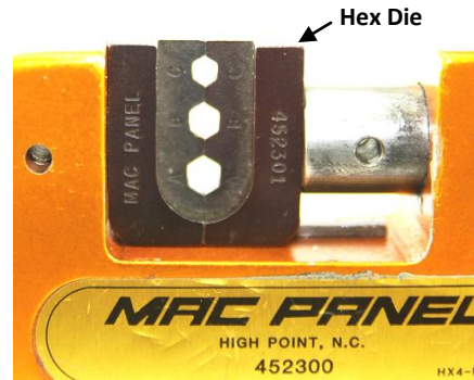
Detail A. (Hex Die 452301 Installed in Crimp Tool)
