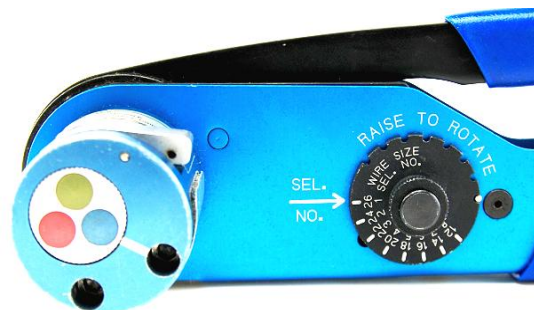
Detail A. (Crimp Tool and Positioner)
