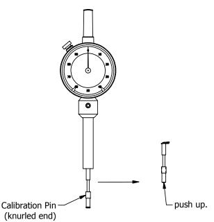
Step 4) With the Calibration Pin firmly seated, Rotate the Depth Gauge bezel until the needle reads " 0 ". Re-tighten the locking screw.
