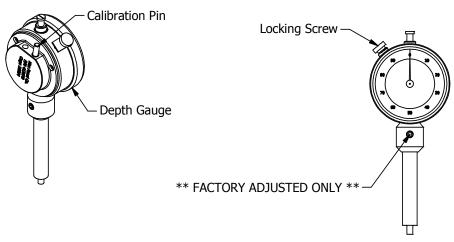
Step 3) Insert the non - knurled end of the Calibration Pin into the end of the Depth Gauge.
