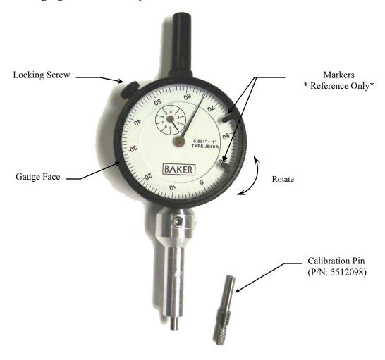
Using the supplied 0.138 diameter calibration pin (P/N 5512098), insert the non-knurled end into the tip at the bottom. Make sure the calibration pin is fully seated, then rotate the dial face until the needle reads "0". Tighten the locking screw. Set the markers at "90" and "70". To use the gauge, push the gauge tip over the coax contact until it is fully seated, avoiding the side of the module. The depth of the center pin is good if the needle is between the two markers.
