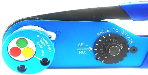
Fig. C. (Positioner inserted into Crimp Tool)
