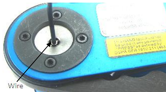
Fig. F. (Stripped wire inserted in Contact)
