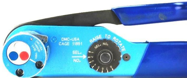
Fig. D. (Positioner inserted into Crimp Tool)
