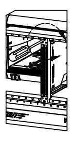
2) To aid in the removal of the DAK / PXI card assembly, the DAK Removal tool can be hooked onto the bottom DAK guide pin. (Detail C)
