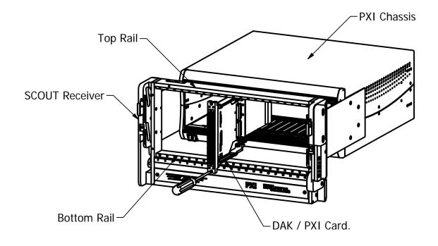
2) Using a 4.5mm flat bladed screwdriver, screw in the BOTTOM DAK screw first (Detail A) This will engage the PXI card into the chassis backplane.
