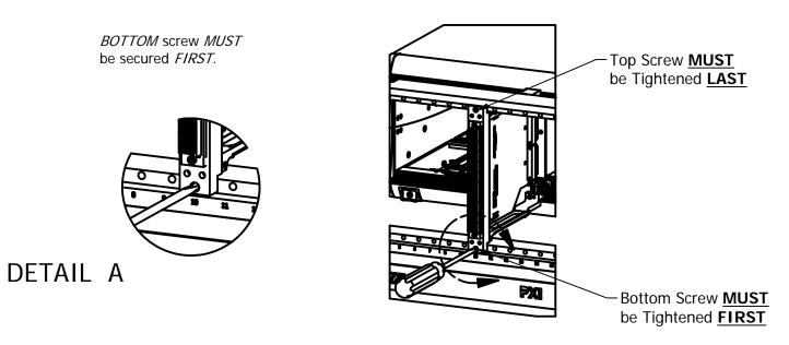
Your DAK / PXI card assembly is now correctly installed in the SCOUT receiver and PXI Chassis.
